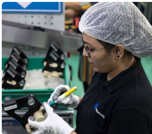
Final inspection of rear-caliper assembly at the disc-brake plant, Chh. Sambhajinagar.
