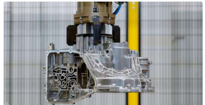
↑ Loading operation on transmission housing line at Endurance SpA plant, Italy
