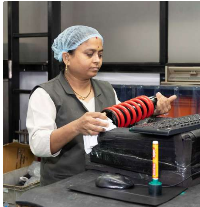
Final inspection of mono-shock assembly, Chh Sambhajinagar
